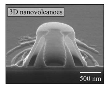
Cross-section of a nanovolcano carved using UV light. The Nanovolcanoes have precisely measured hollow cores and openings at their "mouth," which make them a good candidate for drugdelivery mechanisms, its developers at North Carolina State University say. Courtesy of Chih-Hao Chang, NC State.
